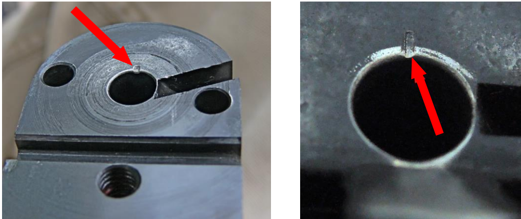
Fig 55 - Damage to chamber caused by firing .22 rifles without a round in the chamber.
