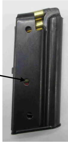
Fig 59 - Rounds loaded correctly
