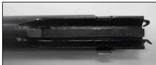
Fig 42 - "W" Cut and Extractor
