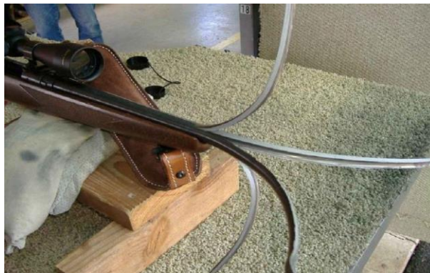
Fig 9 - The end result of barrel obstruction
