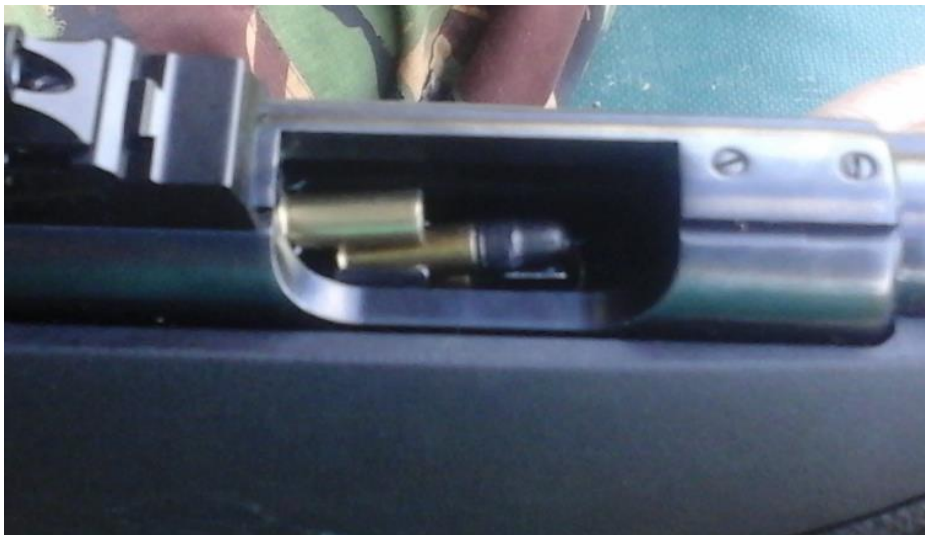
Fig 60 - Spent cartridge fails to eject causing an obstruction
