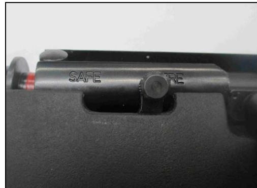
Fig 40 - Safety catch (fire)
